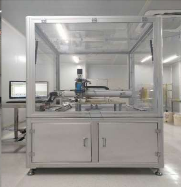
Fiber Laying Machine
