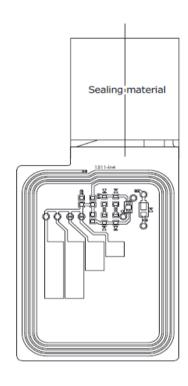
Tolerances of dimensions are ±0.3mm OLED panel thickness is 0.3±0.1mm
