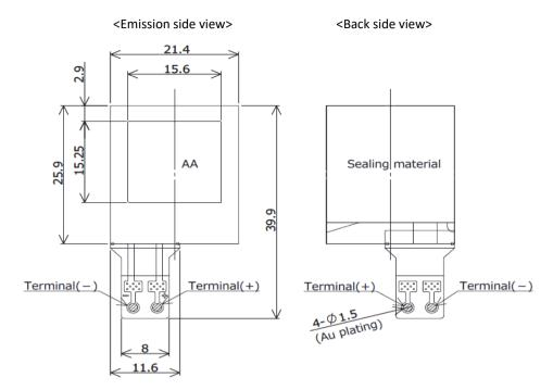
Tolerances of dimensions are ±0.3mm OLED panel thickness is 0.3±0.1mm
