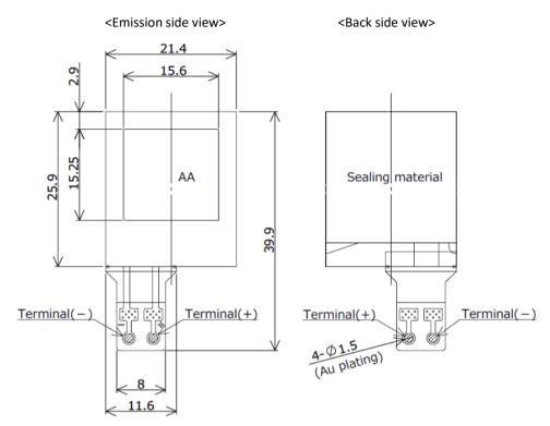
Tolerances of dimensions are ±0.3mm OLED panel thickness is 0.3±0.1mm
